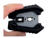
The MTP<sup>®</sup> Pro Field Tool features two ports one for changing the polarity of the connector, the other to change the gender of the pins. Both procedures can be carried out without the removal of the connector's housing.
