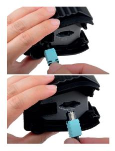
Polarity reconfiguration can be carried out quickly and easily at any time using the MTP<sup>®</sup> Pro Field Tool. The tool has two ports; position the tool so that the word 'Polarity' is facing towards you.
