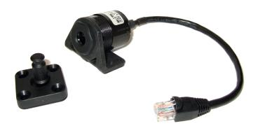
The TZ Radial<sup>™</sup> locking device can be operated via a range of triggers, including internal sensor, push button, contact closure, or RS-485 serial communications network command. The device features a manual override and one-foot cable with an RJ-45 coupler for connection to standard patch cables.
